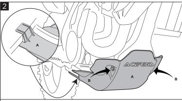
Mount the skid plate (A) fixing the two original screws (B), as shown in the
